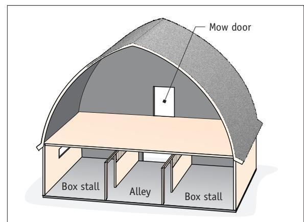
**Figure 3-8** Gothic roof. Two rows of stalls serviced from center alley. Mow over (clear span, laminated rafters).
