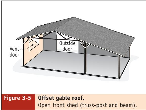
**Figure 3-5** Offset gable roof. Open front shed (truss-post and beam).
