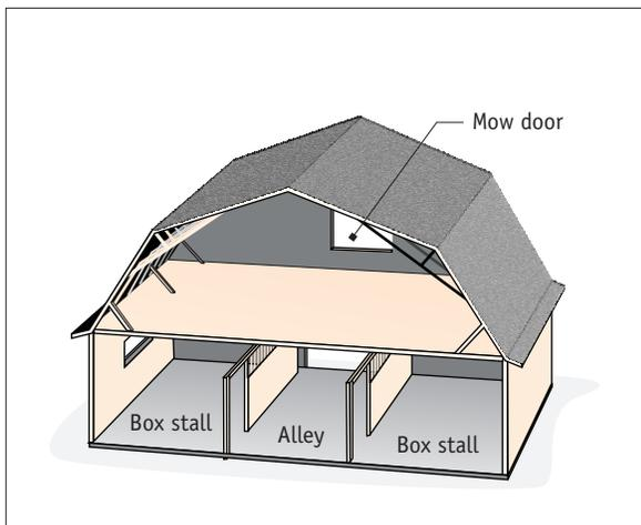
**Figure 3-6** Gambrel roof. Two rows of stalls serviced from center alley (clear span, braced rafter).
