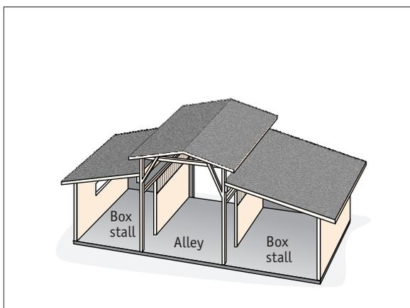
**Figure 3-7** Monitor roof. Two rows of stalls serviced from center alley. (post and beam).
