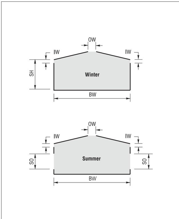
Figure 7. Configurations of natural ventilation openings.
