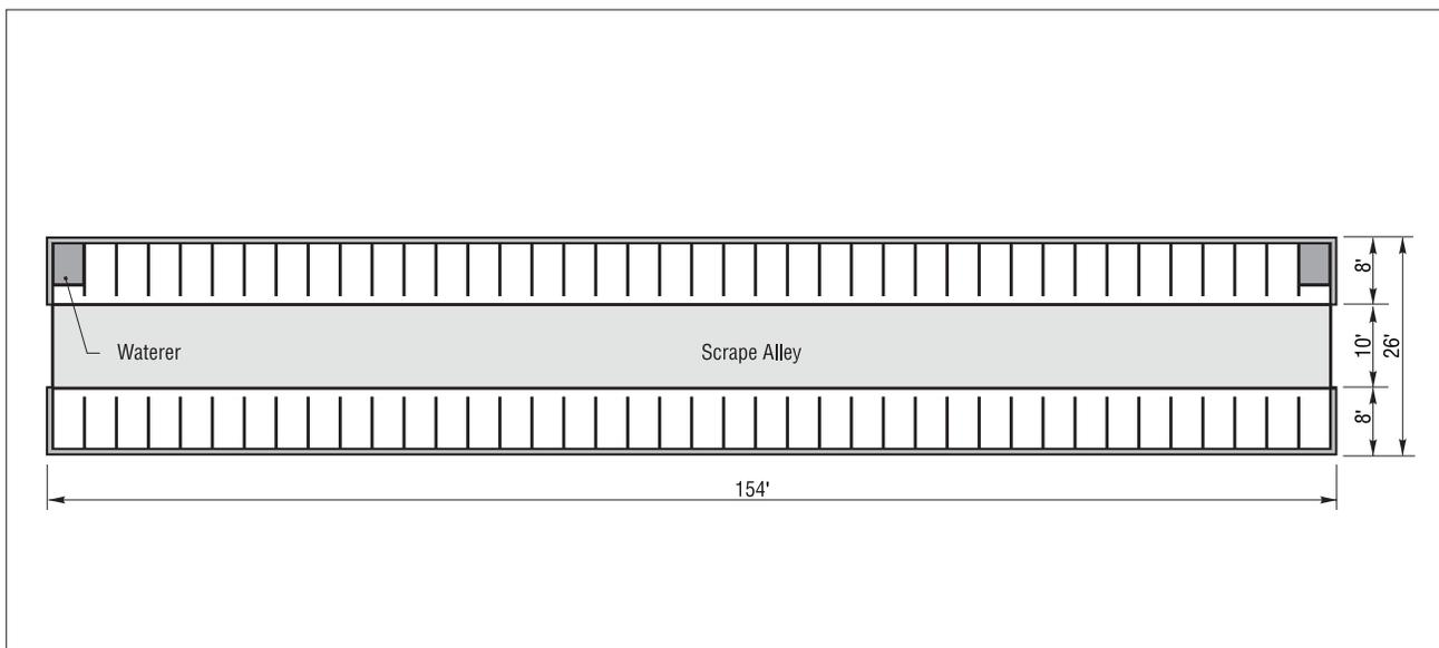
**Figure 9. Example layout for a 26 ft x154 ft building**
