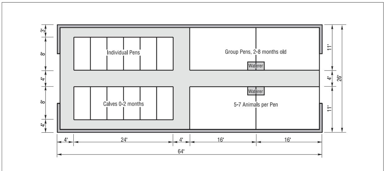
**Figure 8. Example layout for a 26 ft x 64 ft building.**
