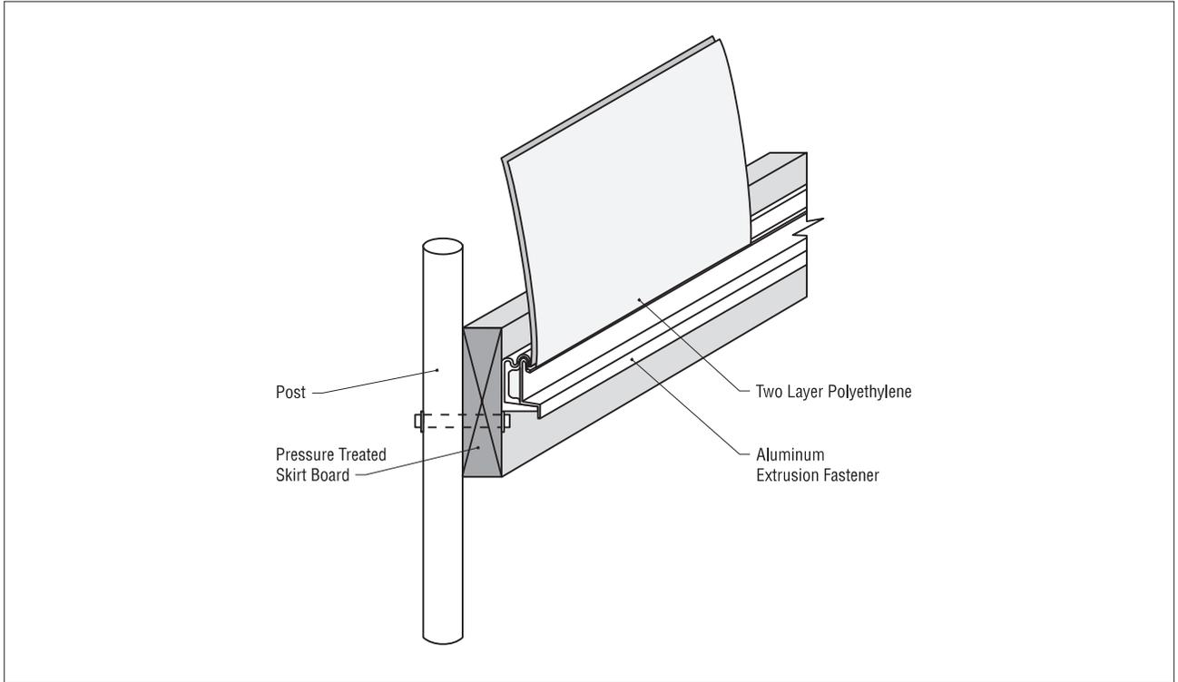
Figure 5. Common method of anchoring plastic covers.
