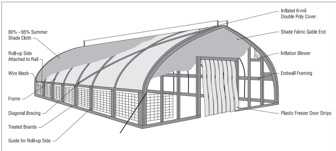
**Figure 1. Basic components of a greenhouse barn**
