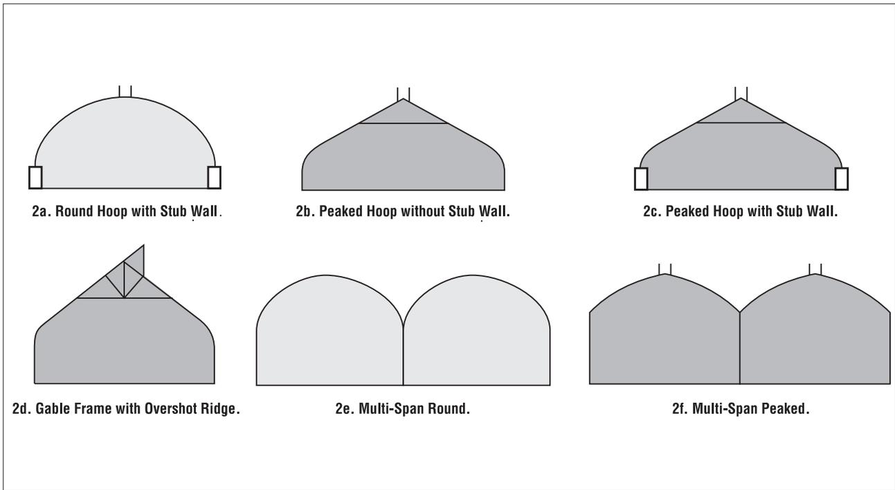
Figure 2. Typical greenhouse frames.
