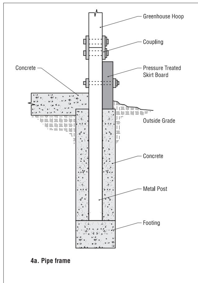
Figure 4. Frame foundation connections.
