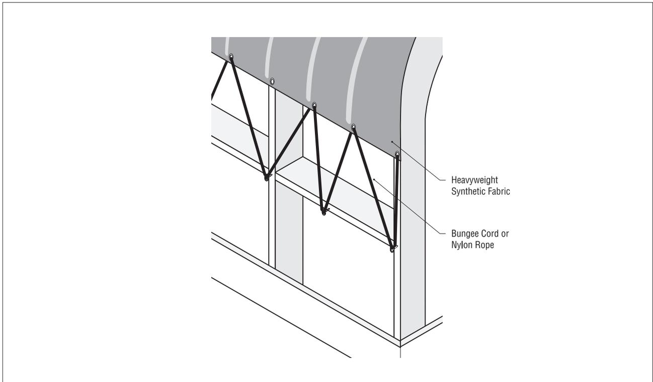
**Figure 6. Common method of anchoring heavyweight synthetic fabrics.**
