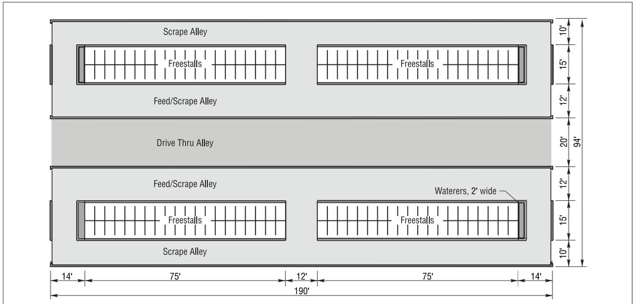
**Figure 10. Example layout for a 94 ft x190 ft building.**
